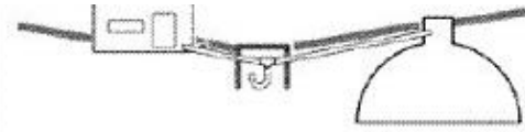
Figure 28: Wherever condensation water cannot drain back into the digester, a water trap becomes necessary Source: TBW
